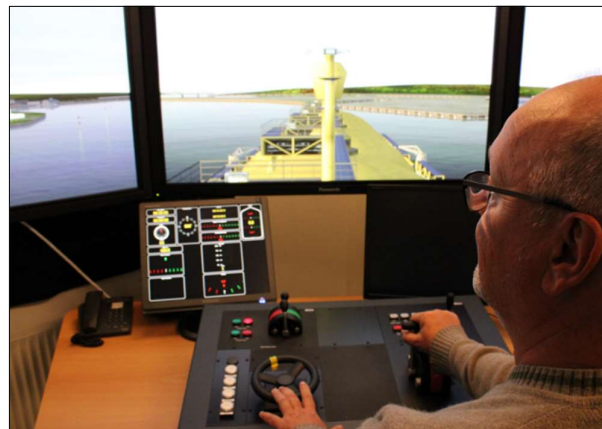
Figure 4 Multi-display system outside view and external handle box
